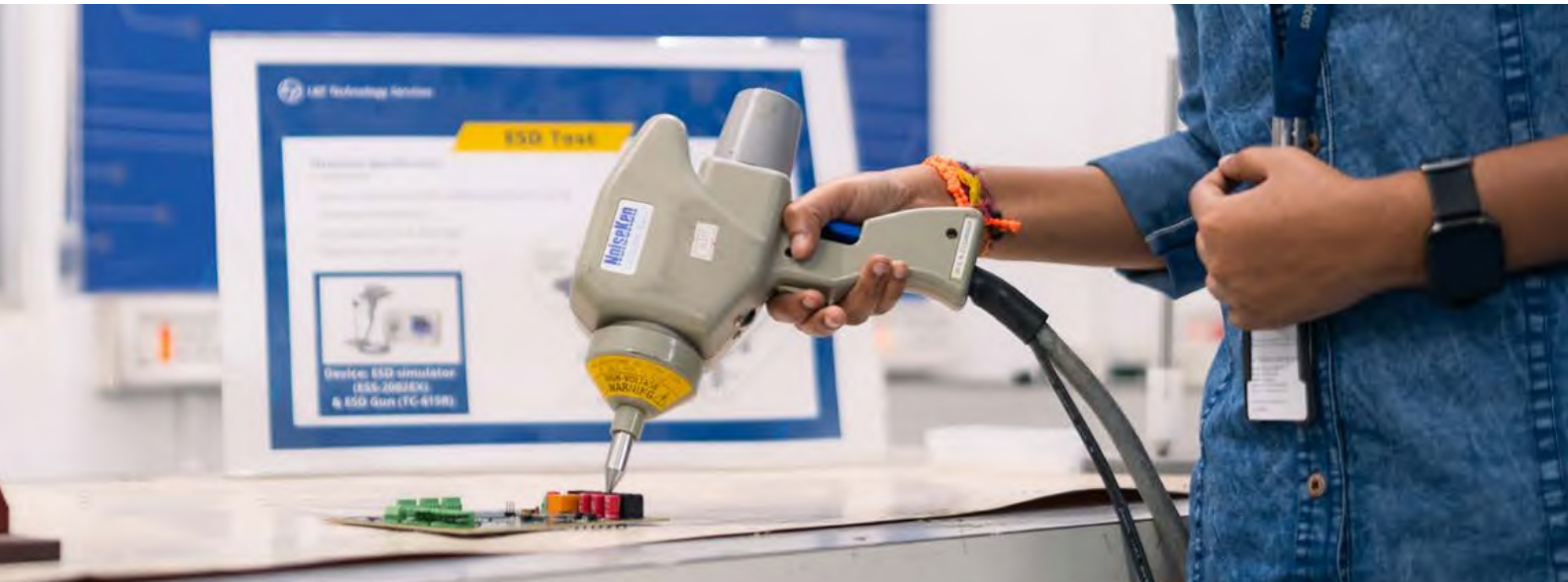
Hands-on EMI evaluation in the lab situated at LTTS Mysuru
